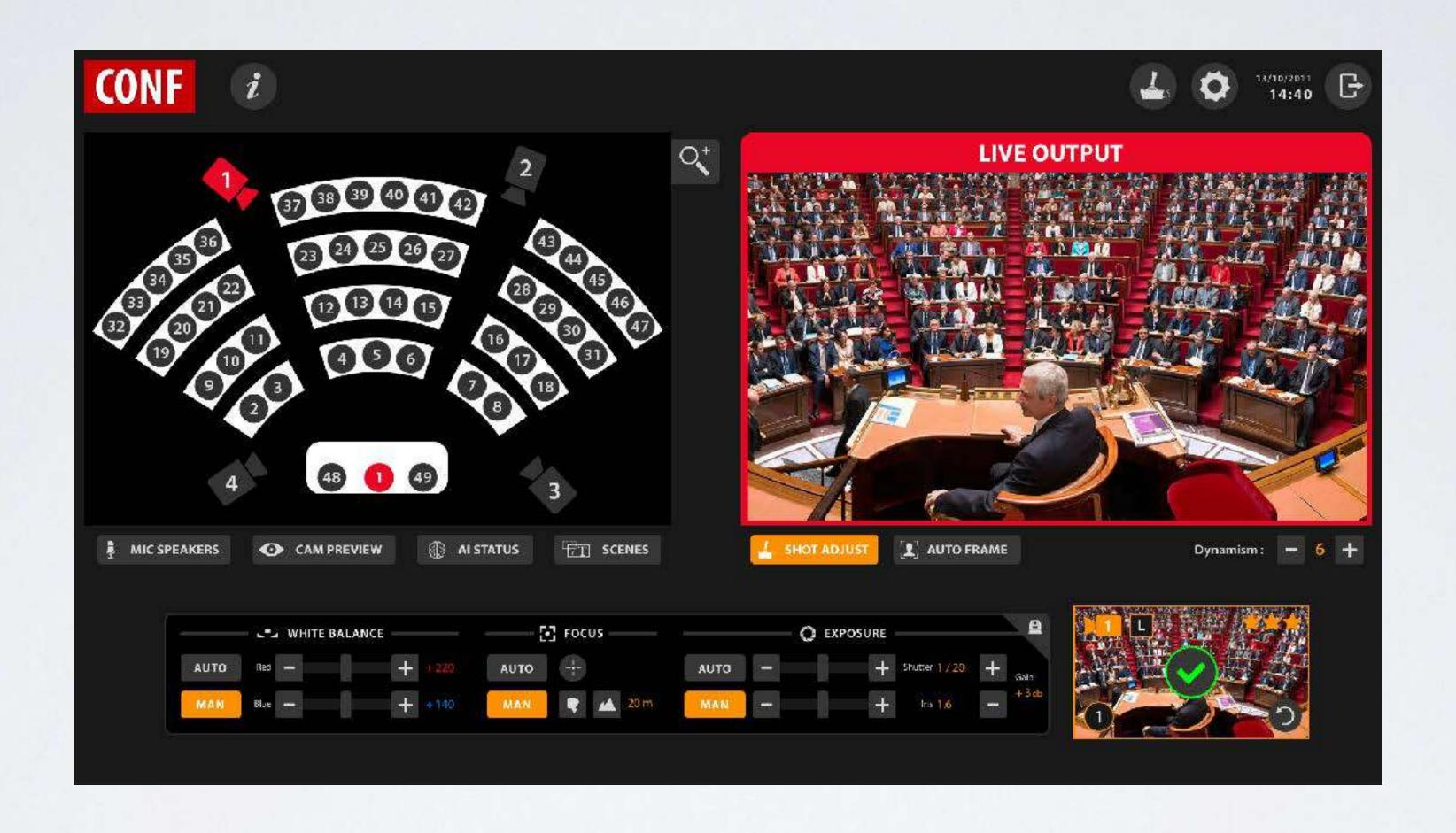
Each microphone is covered by different angles of shots with the PTZ cameras installed in the conference room.
